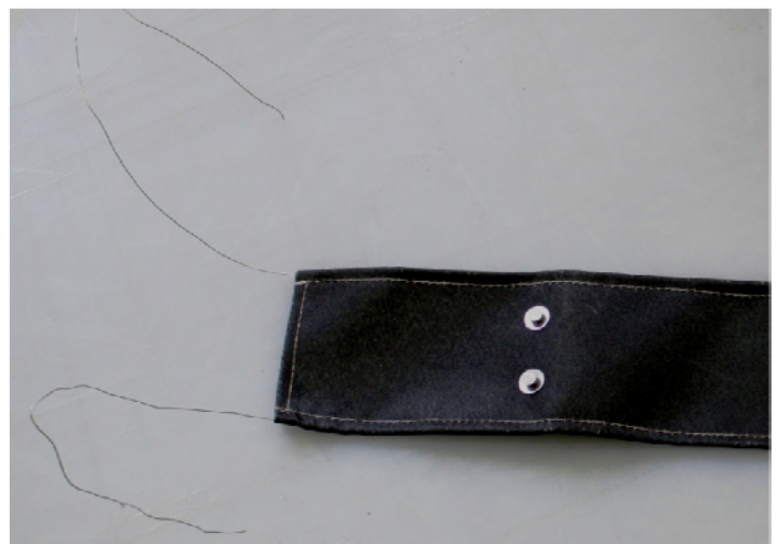
Metal Wires sewn into seam of “seal”
